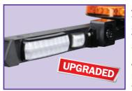
All utility bars come fitted standard with Slimline L.E.D Stop/ Tail/Indicator and Supplementary Reverse Lamps. Multi-voltage, virtually unbreakable polycarbonate lenses and low current draw
