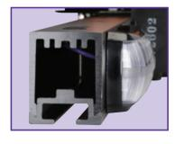
Unique 'Serviceable' two piece anodised extrusion allows the bar to be separated. This provides access to the internal wiring harness and the ability to replace components. T-Slot mounting system allows quick fitting and easy adjustment
