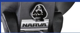
Integrated DT connector & aluminium crush tube
